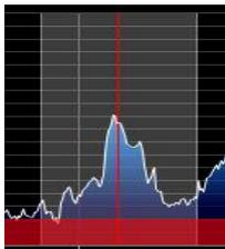
The vertical red line in the center of the RF spectrum windows shows which frequency is currently tuned the receiver. The inside of the gray rectangle is the active bandwidth (or BW) that can be changed by simply dragging the left/right side of the rectangle.
