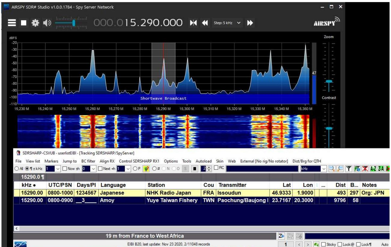
In this screenshot, a Spy Server Network is used to verify a broadcaster on 19-meter. By enabling the "Track mode" option, the first line appears in CSVUB with its transmission highlighted. For very
