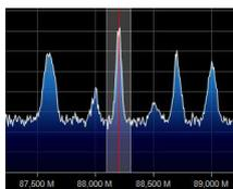
In this window the RF Spectrum is shown visually as a real-time graph. The active signals appear as peaks of greater or lesser intensity. The lower part represents the "noise floor. *A recently introduced feature is the "peak Color" which is activated by clicking with the right mouse button on the Spectrum window, where a yellow line of persistent memory relative to the received signals will appear. It is possible to modify the color by changing the following line:*
