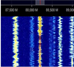
This window shows the graphic representation in real time of the intensity of the received signals as a function of frequency (on the horizontal axis) and time (vertical axis) with the new data represented in cascade starting from the top and going down: hence the name waterfall.
